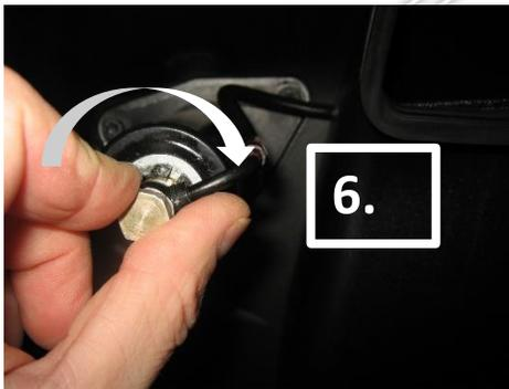
6. During the installment, you can twist the connectors on the bottom of the rams with hand to bring hydraulic lines in a good position.
