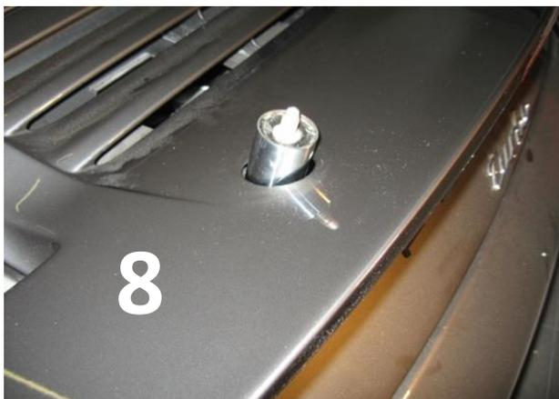
8. continue turned with the hook wrench in clockwise direction to remove the rear lid.
