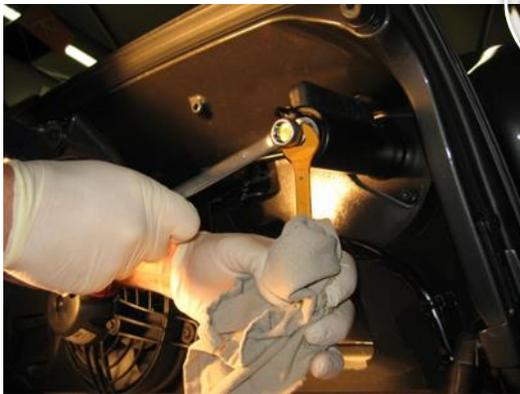
Disconnects oil lines from the rams with the buffed key No. 12 and trapping oil on .( if spoiler total out do it in several steps on left and right ram to prevent damage to hydraulic rams and spoiler fastening)
