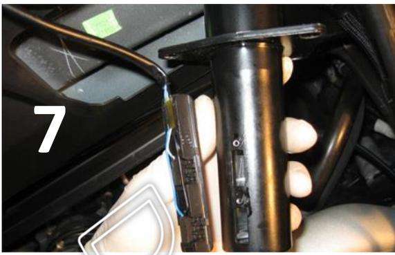
7. Remove micro switch holder from ram and then remove the left hydraulic cylinder from rear lid
