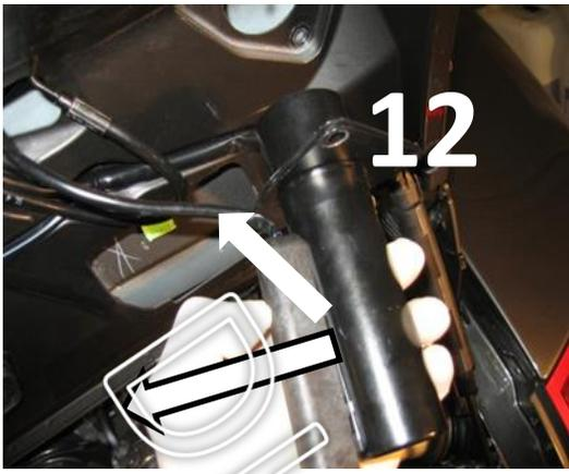
12. unscrew fastening screws from hydraulic cylinder with micro switch to rear lid and remove. Remove plastic cover from micro switch holder.
