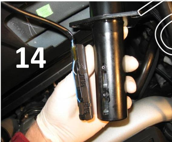
14. Remove micro switch holder from ram and then remove the left hydraulic cylinder from rear lid
