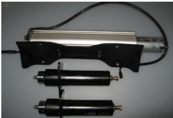
For a good repair service we need complete mechanism. This allows to do a proper checkup and to fill the oil without air bubbles.
