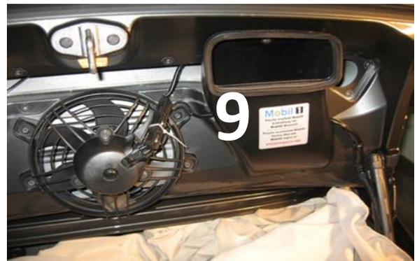
9. installing fan with fan housing. Attach with plastic strip the micro switch holder to fan housing.
