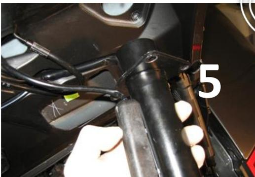
2. disconnect plug connection on fan
