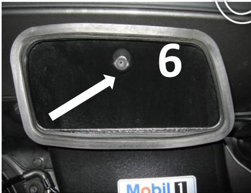
6. Remove air guide : Push the inner plastic part out with the small screwdriver of 3 mm thickness or nail and find this inner part back for further mounting
