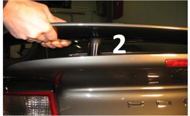
1. Extend the spoiler to its maximum with the switch in the car
